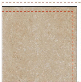
Fig. 1. Caliber range of a tile is the allowable variation from its average facial dimensions.
