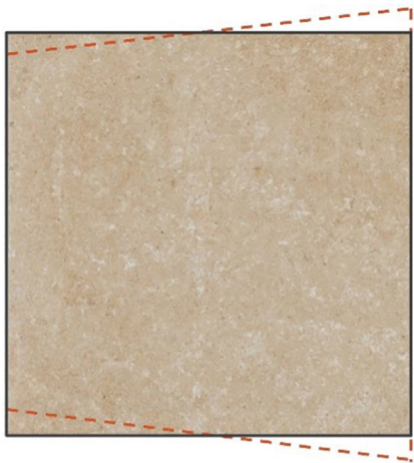
Fig. 5. Wedging tolerances address the allowable variations in length of opposite edges.
